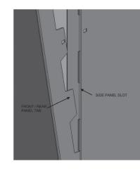
5. Insert the fingers on the bottom of the side panels through the slots in the base panel. Lift up the front
